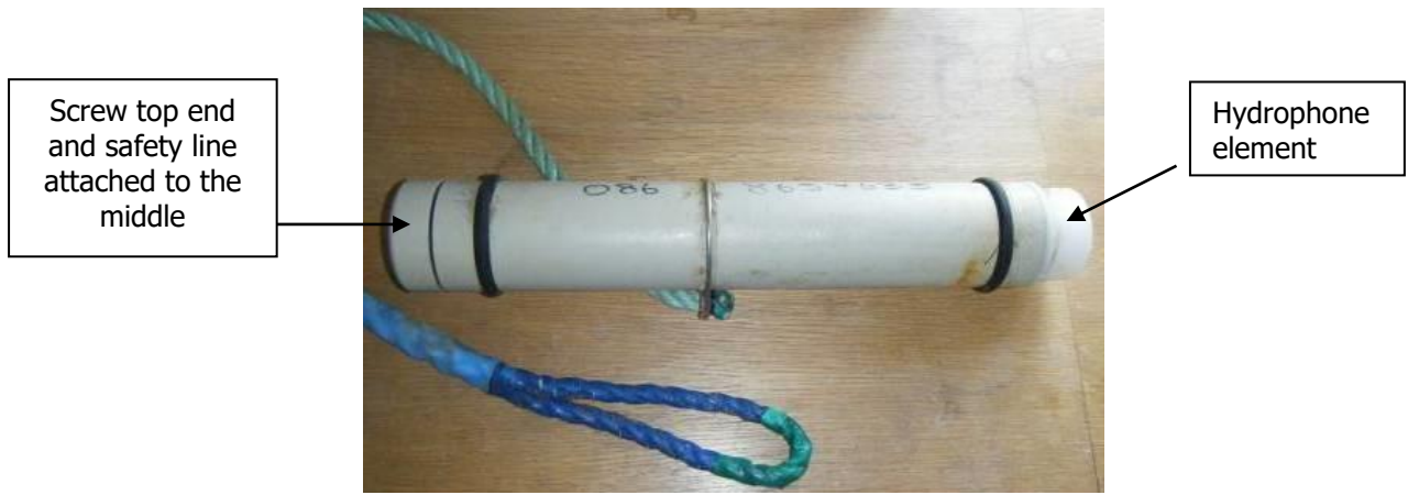
Figure 9: C-POD unit by Chelonia Ltd
